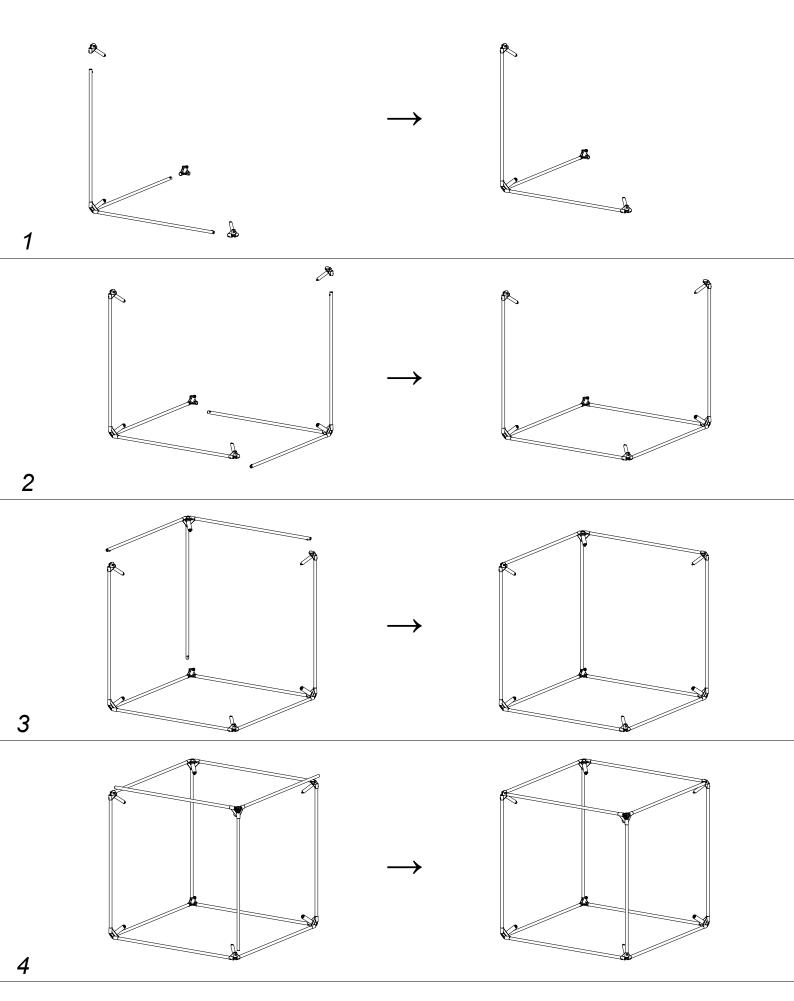
To assemble the cube, use connectors to connect four modules that include three edges of the cube.
